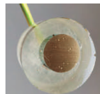
Figure 2. Preparing samples for EIS. Soaking and draining of oil (left). Sample before test, some particles remain in the oil film. The presence of these impurities has been shown to affect the reproducibility of EIS measurements (center). EIS cell (right).
