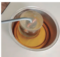
Figure 2. Preparing samples for EIS. Soaking and draining of oil (left). Sample before test, some particles remain in the oil film. The presence of these impurities has been shown to affect the reproducibility of EIS measurements (center). EIS cell (right).
